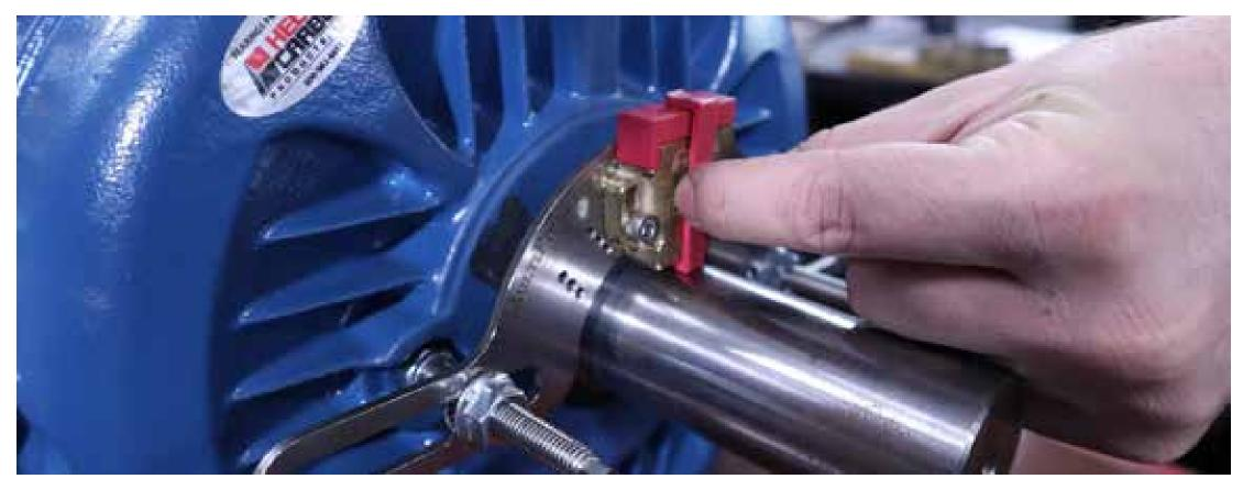
Pull red retainer clip and rotate shaft manually to ensure brush does not contact the keyway and that the entire brush thickness is in contact with the shaft.
