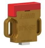
We recommend the brush ride perpendicular to the shaft. The track in which the brush rides on the shaft should be free of scratches, nicks, dents, or defects of any kind. Ideally the shaft surface should be clean with a surface finish within the standard range of most motor manufacturers of 8 to 63 RMS. Do not use any external lubrication. The brush will supply its own lubrication.
