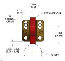
2. **Attach** holder to unit using two 4-40 or M3 screws.
