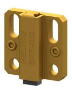
The BPK-IM2 Bearing Protector Kit is mounted using two 4-40 screws (included) or 3 mm screws (not included). The holder should be mounted 0.090" to 0.125" (2.3 mm to 3.2 mm) from the shaft.
